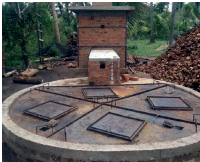
Haritha Angara Environment friendly closed charcoaling pit
