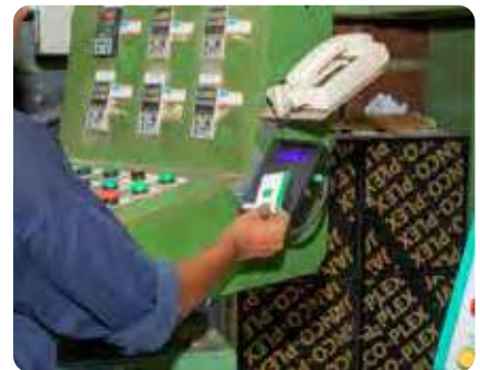
Smart machine parameter monitoring system implementation for TY 03 and TY 04 machines
