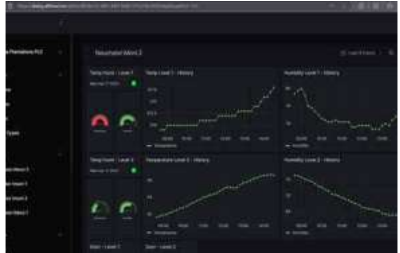
IoT Temperature Monitoring System for Drying Towers
